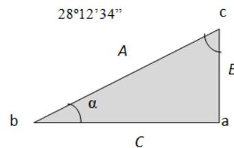
$$\begin{aligned} \operatorname{cos} \alpha &= C / A \rightarrow C = A \operatorname{cos} \alpha \\ C &= 15 \text{ cm} \cdot \operatorname{cos} 28^\circ 12' 34'' = 13,22 \text{ cm} \end{aligned}$$
